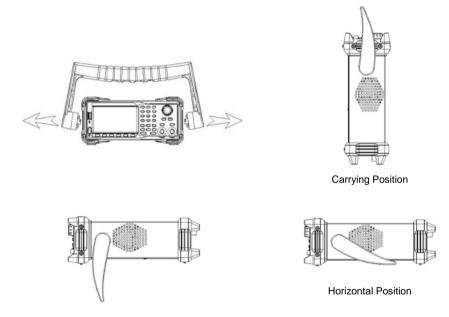
Figure 1 Adjust the Handle
