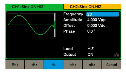
Then press the corresponding softkey to select the desired unit. For example, press **kHz**.
