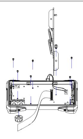
6. Remove the keypad circuit board assembly.
