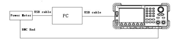
3. Select Sine waveform of the generator and set the amplitude to 1 V and 2.5 V, frequency to the values listed below in sequence.
