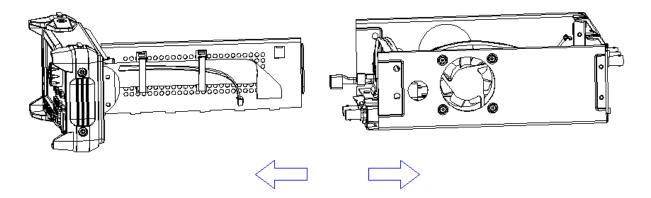
5. Pull out the knob and then remove the screws attaching the hardware partition plate and the front cabinet screws.
