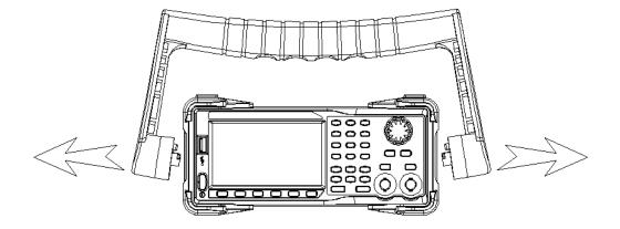
2. After removing 4PCS screws of the pad and 1PCS screw at the bottom of the generator's case, remove the metal shell carefully from the main body to avoid being scratched.
