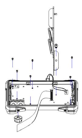
6. Remove the keypad circuit board assembly.
