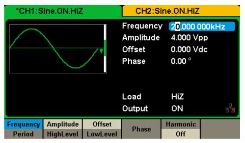
**Note:** The desired numerical value can be modified using the knob and direction keys.
