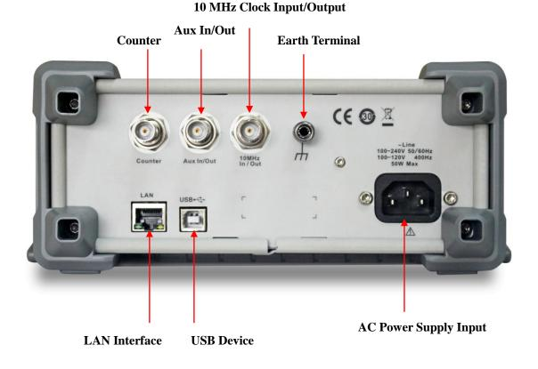
**WARNING:** For protection from electric shock, the grounding power cord must not be defeated. If only a two-contact electrical outlet is available, connect the instrument's chassis ground screw (see above) to a good earth ground.
