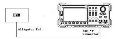
3. Select Sine waveform of the generator and set the amplitude to the values listed below in sequence.
