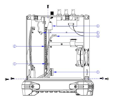
4. Separate the front panel from the main body of the generator.
