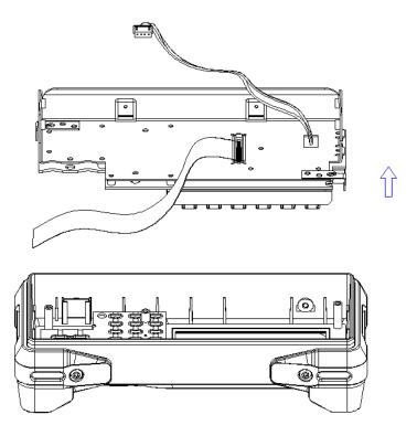
7. Remove the 3PCS screws holding the screen bracket and remove the
