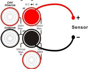
Diagram 2-28 Sketch Map for Measuring Temperature
