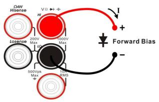
Diagram 2-26 Sketch Map for testing Diode
