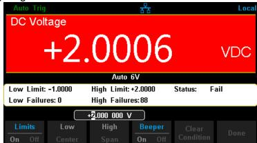
Diagram 3-10 Limits Test Result
