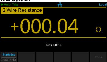
Diagram 3-3 Test Lead Impedance
