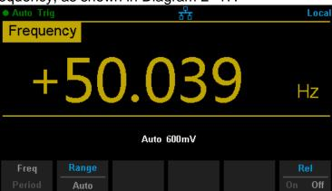
Diagram 2-19 Frequency Measurement Interface
