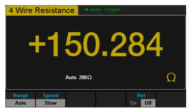
Diagram 2- 15 4-Wire Resistance Measurement Interface
