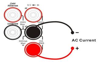
Diagram 2- 12 Sketch Map for Measuring AC Current
