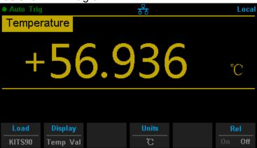
Diagram 2-27 Temperature Measurement Interface
