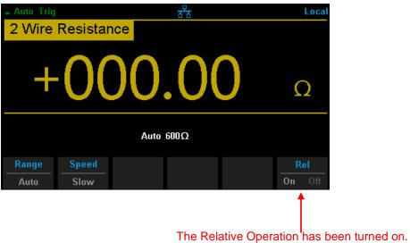
Diagram 3-5 Lead Impedance after Operation
