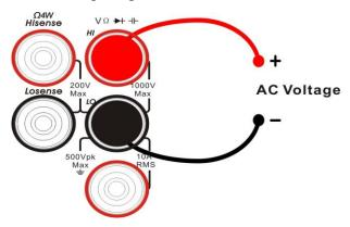
Diagram 2-9 Sketch Map for Measuring AC Voltage
