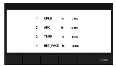
Diagram 2-48 Chip Test Interface
