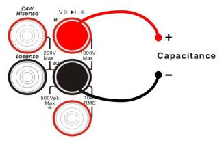
Diagram 2-18 Sketch Map for Measuring Capacitance
