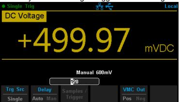
Diagram 2-53 Setting interface of Auto Trigger
