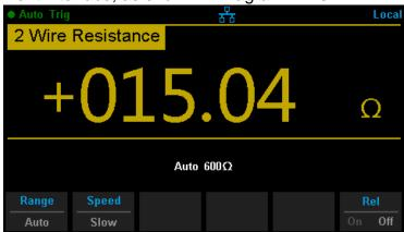
Diagram 2-13 2-Wire Resistance Measurement Interface
