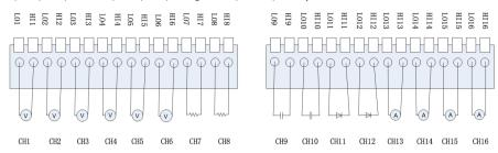
Remarks: [1] CH1 to CH12 can be used to measure DCV /ACV/ 2WR/ 4WR/ CAP/ FREQ/ DIODE/ CONT / TEMP. CH13 to CH16 can only be used for current measurements, less-than 2.4A
