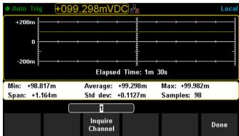
Set the [Inquire Channel] by direction keys and the interface displays the minimum, average, maximum, span, standard deviation, samples and trend chart of measurement results of the setting channel during the scan operation.
