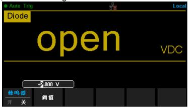
Diagram 2-19 Diode Measurement Interface
