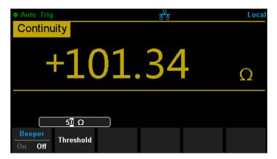
Diagram 2-7 Set Up the Short-circuit Resistance
