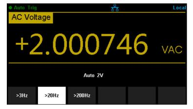
Diagram 2-6 AC Filter setting interface
