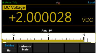
Diagram 2-48 Bar Meter Display Mode
