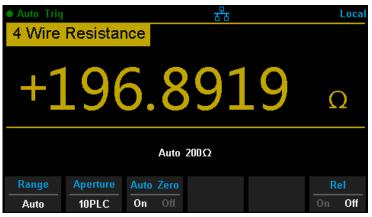
Diagram 2-14 4 Wire Resistance Measurement Interface
