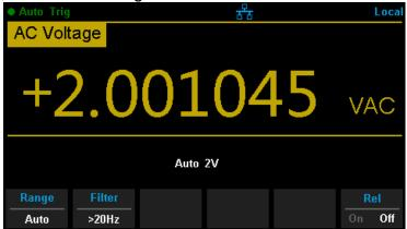
Diagram 2-11 AC Voltage Measurement Interface
