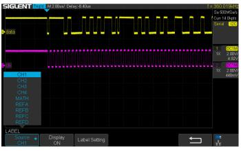
When multi-channel measurement is used, corresponding labels are set for different sources to facilitate observation and reading.
