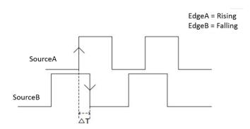
Click the SourceB Setting region to set the edge trigger source, threshold, and slope.
