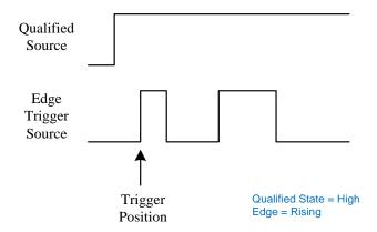
When the type is "Edge", the oscilloscope triggers at the first edge after the specified edge (Rising or Falling) of the qualified source; when the type is "Edge with Delay", a time limit condition is available.
