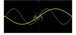
Pinch and spread the waveform horizontally to re-scale the timebase
