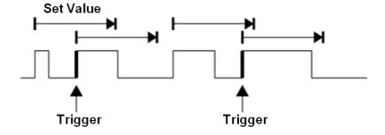
Trigger source, slope (rising, falling), limit range, and time value can be set in the trigger dialog box. Holdoff, coupling, and noise reject can be set in interval trigger, see the sections "Holdoff", "Trigger Coupling" and "Noise Reject" for details.
