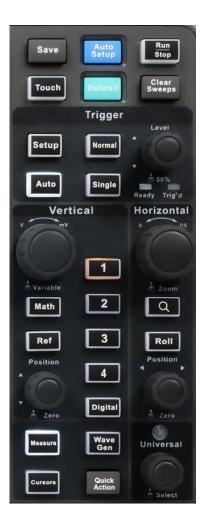
The front panel is designed to operate the basic functions without having to open the software menu. Most of the front panel controls duplicate functionality available through the touch screen display but the operation is more quickly achieved.
