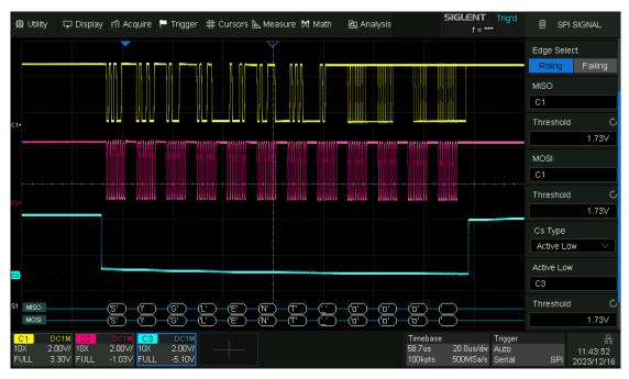
When the CS type is set to CLK Timeout, turn on Cursor, measure the clock idle time between frames as 505 us, and measure the interval between clock pulses as 0.5 us, then set the timeout to a value between 0.5 us and 505 us. In this example it is set to 4.5 us:
