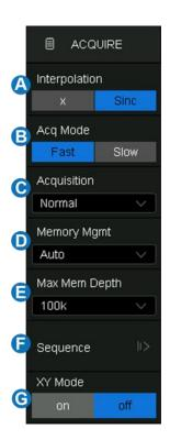
**Interpolation** -- At small timebase settings, the number of original points on the screen may be less than the number of display pixels in the grid area, so interpolation is necessary to display a continuous waveform. For example, at 1 ns/div timebase and 2 GSa/s sample rate, the number of original points is 20, but the grid area includes 1000 horizontal pixels. In this case, the oscilloscope needs to interpolate the original points by 50.
