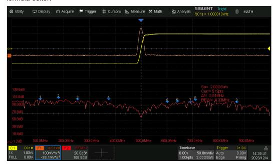
In this example, F1=d (C1)/dt and F2=FFT (d (C1)/dt) are equivalent to F2=FFT (F1), which is equivalent to performing FFT analysis on the differential operation results of C1 waveform.
