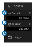
**Note:** The low and high current values are used to calculate the trigger level and adjust the oscilloscope vertical scale. After the load changes, the current value changes from low to high (or from high to low), and the oscilloscope triggers and performs to measure the transient response stability time.
