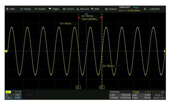
Fixed delay, timebase is changed to 100 ns/div, the value of X cursors (-50 ns, 100 ns) remains fixed. The grid number of X cursors is changed to -0.5div, 1div.
