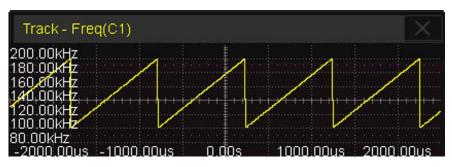
The upper limit of the statistic number in a frame is set in Statistics Setting > AIM Limit , which means the values exceeding the limit will not be shown in the track plot.
