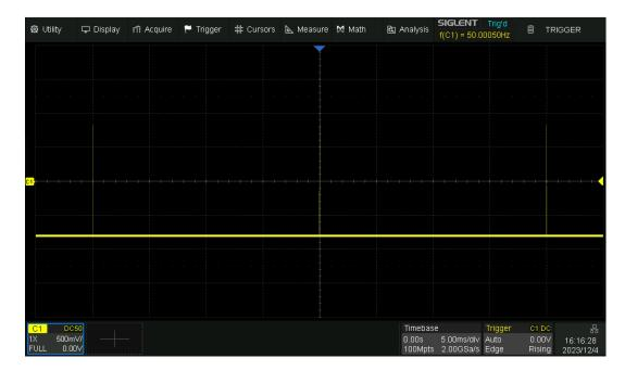
In normal mode, 3 pulses can be obtained on the screen with the sample rate of 2GSa/s at the maximum memory depth.
