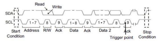
**10 Address & Data** — If all bits match, then trigger on the Ack bit followed by the Data. Frame (Start: Address 1st byte: R/W: Ack: Address 2nd byte: Ack: Data)
