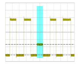
First, set the trigger type to Runt to trigger on the dwarf pulse. See the section "Runt Trigger" for details.
