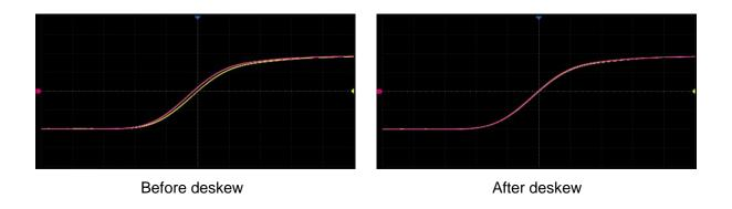
**Note:** When the channel with deskew compensation is the trigger source, the trigger delay indicator does not change as the deskew value changes.
