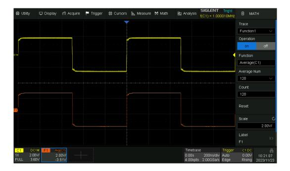
**ERES** -- Reduce bandwidth random noise on the measured signal and improve signal-to-noise ratio by filtering the sampling points
