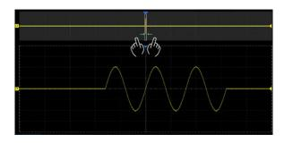
Adjust the horizontal/ vertical scale of the main window by using a pinching or spreading gesture in the gray area of the main window
