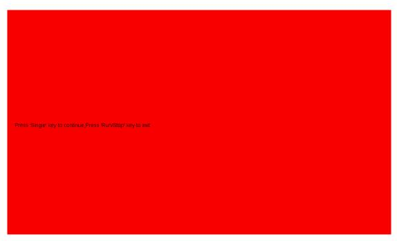
Press the "Single" button to switch to green and blue display mode. Observe whether there is any color distortion, bad pixels, or scratches on the screen. Press the "Run/Stop" button to exit the screen test mode.
