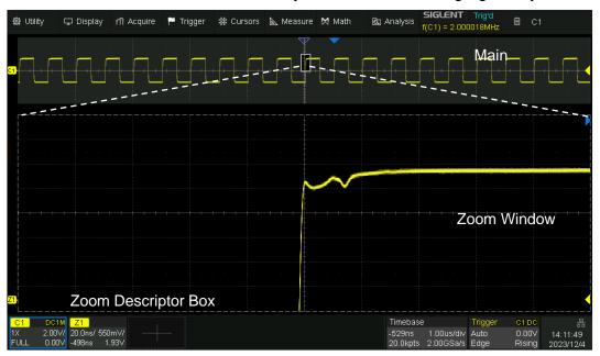
The area not covered by the gray background in the main waveform area is the range to be zoomed in (zoom area). Touch the Zoom Vertical Parameters and Zoom Horizontal Parameters regions shown in the figure above to recall the quick dialogs for setting the vertical and horizontal parameters of the zoom window.
