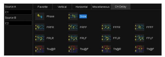
In the parameter selection area, the channel corresponding to Source A is specified first, and then the channel corresponding to Source B . Finally, the measurement parameter is selected. For example, to activate the skew between C1 and C2, you can follow the following steps:
