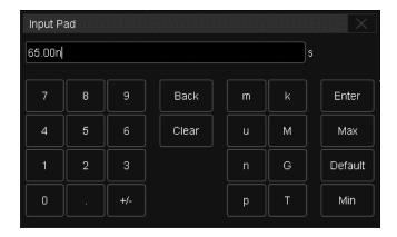
Let's use the operation of setting the "deskew" of a channel as an example: If the expected value is 65 ns, input "65" on the virtual keypad, and then choose the units n to complete the operation. On the virtual keypad, touching the button Max, Min, and Default quickly sets the parameter to the maximum, minimum, and default values.
