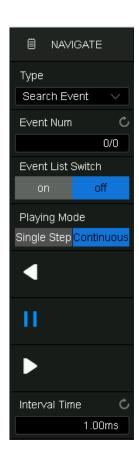
• Touch the Event List Switch area to turn on or off the list. The list contains time labels for each event. Touching a row in the list automatically jumps to the corresponding event. This operation is equivalent to specifying an event in the Event Num area.
