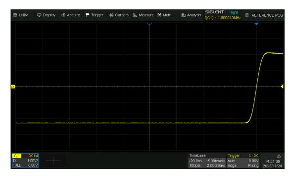
Fixed delay, timebase is changed to 5 ns/div, the horizontal delay value remains fixed, while the grid number of delay changes to 4div
