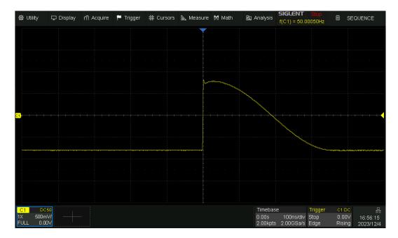
In the example, 45976 pulses can be obtained with the sample rate of 2 GSa/s at the maximum memory depth.
