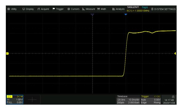
Timebase = 10 ns/div, Horizontal Delay = -20 ns = - 2 div
