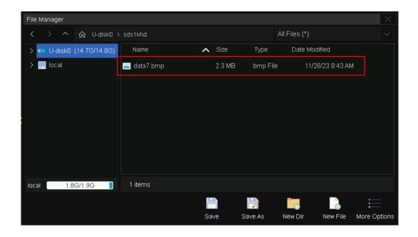
In step 4, if Save is selected instead of Save As , the system saves the file as the default file name SDS1xx4XHD\_BMP\_n.bmp, where n is an integer incrementing from 1. The default save path is \SIGLENT\.
