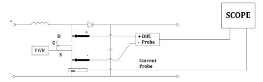
**Note:** Perform a Deskew operation between the voltage and current input channels before the test. See section "Switching Loss" for more details on deskewing.
