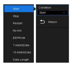
**Start** — The oscilloscope will be triggered when the SDA line transitions from high to low while the SCL is high.
