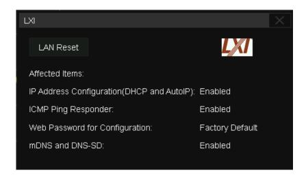
Click LAN Reset to restore the LAN defaults to your oscilloscope. It will enable automatic IP, ICMP Ping responder, and Multicast DNS, and reset the webserver password which is set in
