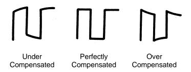
5. Use a non-metallic driver to adjust the low-frequency compensation adjustment hole on the probe until the waveform displayed is as the "Perfectly compensated" in the figure above.
