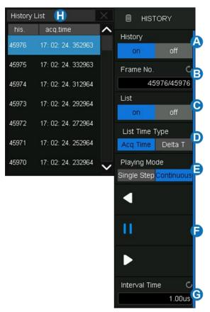
The oscilloscope automatically stores acquired frames. It can store up to 80,000 frames but the number may vary due to the memory depth and timebase settings. Turn on history mode, then the stored frames can be recalled and measured.
