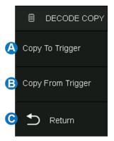
**Note:** The synchronization is not automatic. If the settings at one place change, a copy operation is necessary to re-synchronize.
