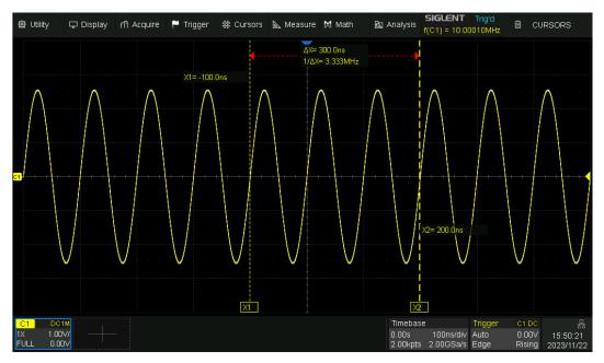
Fixed position, timebase is changed to 100 ns/div, the grid number of X cursors (-1div, 2div) remains fixed. The value of X1 and X2 is changed to -100 ns, 200 ns.
