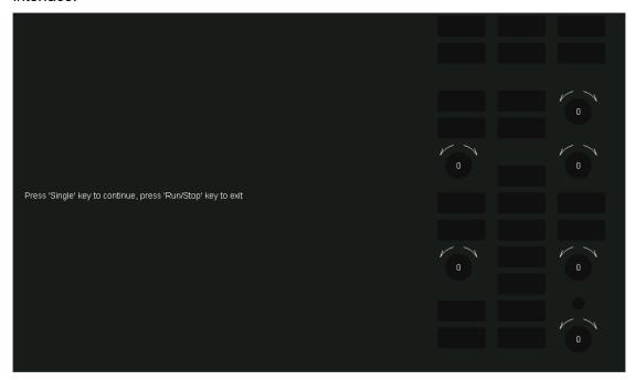
Press the "Single" button and the first LED on the front panel will light. The corresponding position of the key on the screen will also change color. Press the "Single" button to check the next button. Press the "Single" button consecutively until all the backlights are tested. Press the "Run/Stop" button to exit the LED test.
