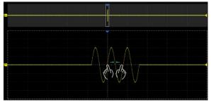
Adjust the horizontal scale of the Zoom window by horizontal pinch and spread in the zoom area of the main window or the Zoom window
