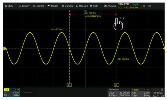
Touch the display area of  $\triangle X$  (or  $\triangle Y$ ) in Following mode and drag it to move the two cursors simultaneously, as shown in the figure below. This is equivalent to the operation on the cursor type X1-X2 or Y1-Y2.
