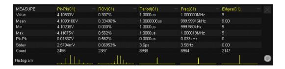
Touch the histogram area of a parameter to enlarge it for details. You can move the large histogram window position around the display by dragging. Touch the histogram of another parameter to switch to the corresponding enlarged histogram.
