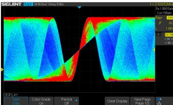
The color temperature display is similar to the intensity-graded trace function, but the trace occurrence is represented by different colors (color "temperature") as opposed to changes in the intensity of one color. Red colors represent events that occur more frequently, while blue is used to mark points that occur less frequently
