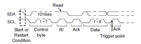
• 7- bit Address & Data Condition — The oscilloscope triggers on a read or write frame in 7- bit addressing mode on the 17th or the 26th clock edge if all bits in the pattern match. For triggering purposes, a restart is treated as a start condition
