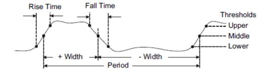
Figure 78 Time Measurements
