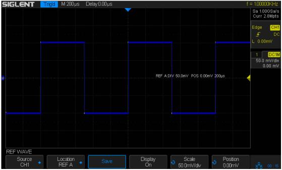
Figure 68 Reference Waveform
