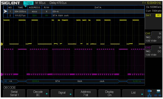
Figure 37 IIC Decode Result
