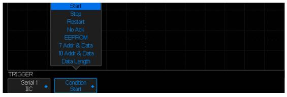
Figure 35 IIC TRIGGER Menu
