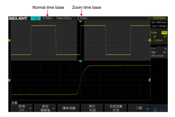
The area of the normal display that is expanded is outlined with a box and the rest of the normal display is ghosted. The box shows the portion of the normal sweep that is expanded in the lower half.
