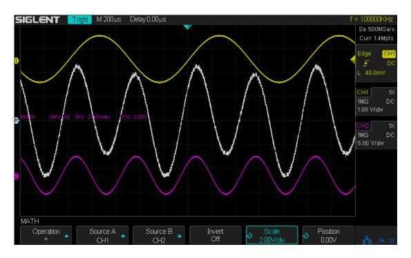
4. If you want to invert the math waveform, press the **Invert** button and set the option to **On** to invert the display of the math waveform.
