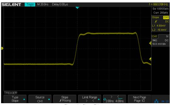
Figure 24 Slope Trigger
