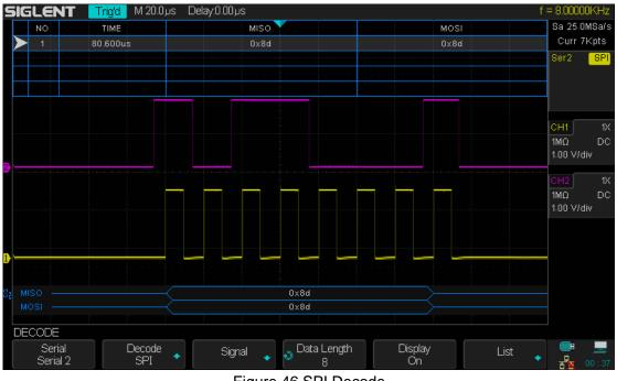
Figure 46 SPI Decode
