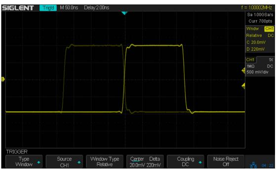
Figure 28 Relative Window Trigger
