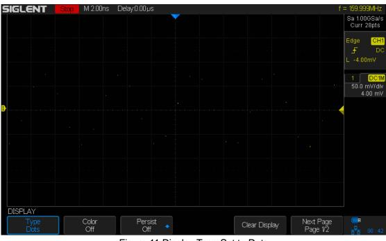
Figure 11 Display Type Set to Dots
