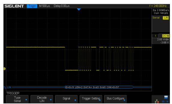
• Data Error — The oscilloscope triggers when detects data error.
