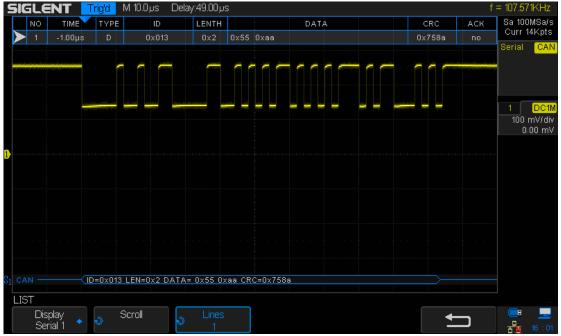
Figure 55 CAN Decode
