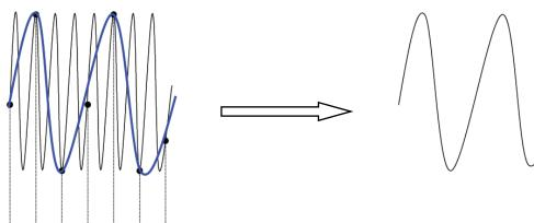
**3. Waveform Leakage:** when the sample rate is too low, the waveform rebuilt from the sample data does not reflect all the actual signal information.
