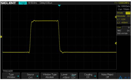
Figure 27 Absolute Window Trigger
