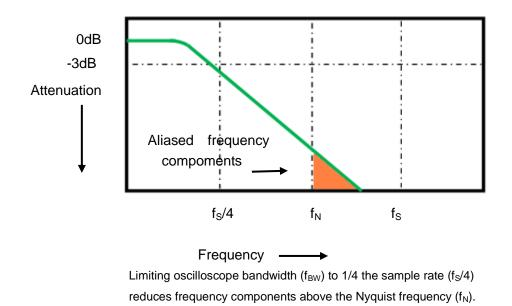
So, in practice, an oscilloscope's sample rate should be four or more times its bandwidth:  $f_S = 4$ fBW. This way, there is less aliasing, and aliased frequency components have a greater amount of attenuation.
