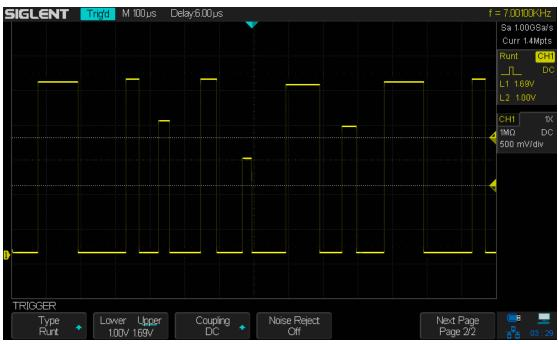
Figure 32 Runt Trigger
