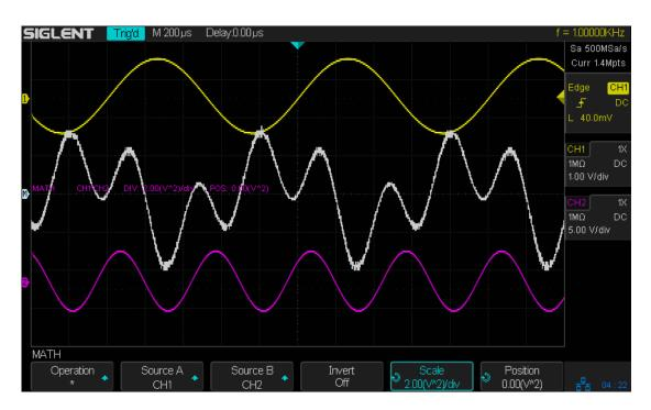
If you want to invert the math waveform, press the **Invert** button and set the option to On to invert the display of the math waveform.
