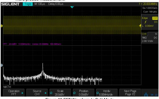
Figure 69 FFT Waveform In Split Mode
