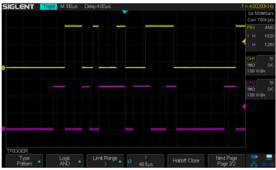
Figure 33 Pattern Trigger
