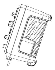
Figure 3 Adjust the Supporting Legs
