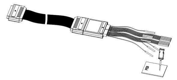
Figure 60 Connect the Digital Probes
