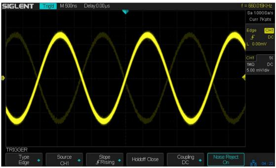
Figure 21 Turn off the Noise Reject
