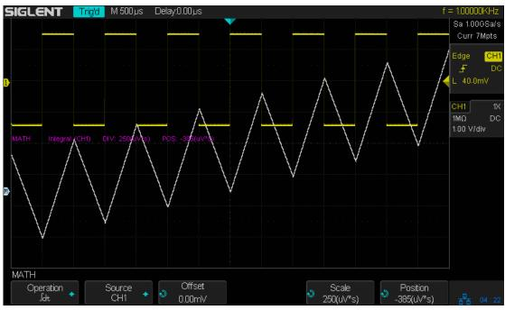
Figure 72 Integral with Offset
