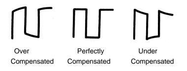
4. Use a nonmetallic driver to adjust the low-frequency compensation adjustment hole on the probe until the waveform displayed is as the "Perfectly compensated" in the figure above.
