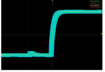
The oscilloscope utilizes a hardware-based Mask Test function, performing up to 14,000 Pass / Fail decisions each second. It is easy to generate user-defined test templates to provide trace mask comparisons, making it suitable for long-term signal monitoring or automated production line testing
