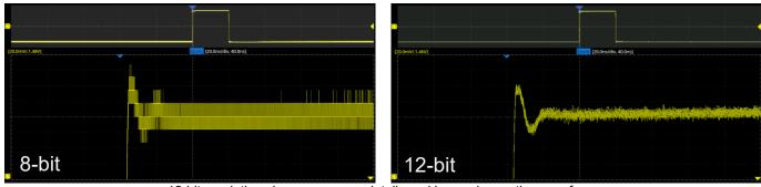
12-bit resolution shows you more details and less noise on the waveform.
