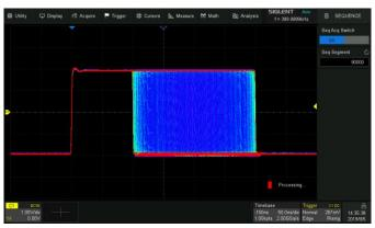
Segmented memory collection will store the waveform into multiple memory segments (up to 80,000) and each segment will store a triggered waveform as well the dead time information. The interval between segments can be as small as 1.12  $\mu$ s. All of the segments can be played back using the History function
