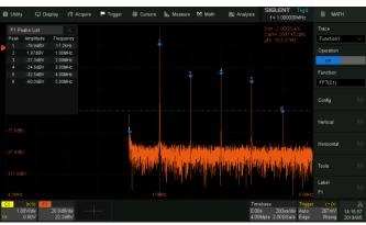
FFT supports up to 4 Mpts operation. This provides high-frequency resolution with a fast refresh rate. The FFT function also supports a variety of window functions so that it can adapt to different spectrum measurement needs. Three modes (Normal, Average, and Max hold) can satisfy different requirements for observing the power spectrum. Auto peak detection and markers are supported.
