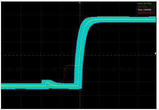
The oscilloscope utilizes a hardware-based Mask Test function, performing up to 28,000 Pass / Fail decisions each second. It is easy to generate user-defined test templates to provide trace mask comparisons, making it suitable for long-term signal monitoring or automated production line testing
