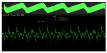
Using hardware-based Zoom technique and record length of up to 400 Mpts, users can select a slower timebase without compromising the sample rate, and then quickly zoom in to focus on the area of interest
