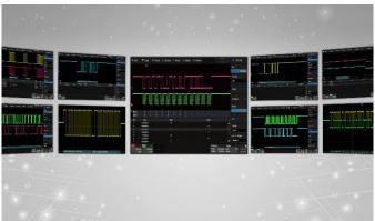
Display the decoded characters through the events list. Bus protocol information can be quickly and intuitively displayed in tabular form. I<sup>2</sup>C, SPI, UART, CAN, LIN, CAN FD, FlexRay, I<sup>2</sup>S, MIL-STD-1553B, SENT, Manchester and ARINC429 are supported
