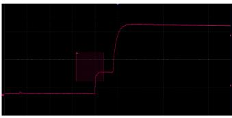
Zone Trigger is available for advanced triggering. Combine spatial triggering with common trigger modes to isolate signals of interest
