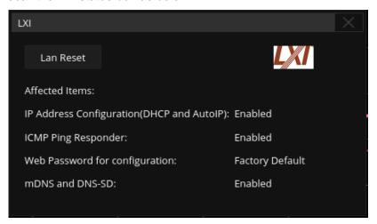
Touch LAN Reset to restore the LAN defaults to your oscilloscope. It will enable automatic IP, ICMP Ping responder, and Multicast DNS, and reset the webserver password which is set in
