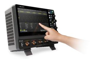
Waveforms, cursors, and trigger levels can be adjusted and a rectangular zone can be drawn by touch gestures in the grid area.
