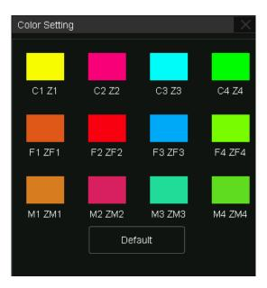
Select a color directly on the palette and preview its hue, saturation, light, and RGB values or directly modify the color parameters to customize the color. After the change, touch OK to confirm.
