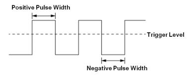
**Less than a time value (≤)** -- Trigger when the positive or negative pulse time of the input signal is lower than the specified time value. Below is an example of a trigger condition set to a positive pulse width < 100ns.
