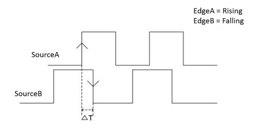
Touch the SourceB Setting region to set the edge trigger source, threshold, and slope.
