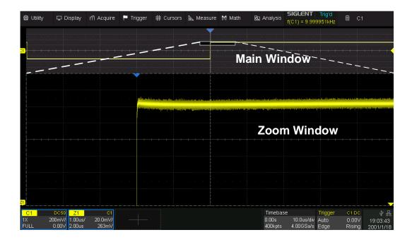
The area not covered by the gray background in the main waveform area is the range to be zoomed in (zoom area). Click the descriptor box of the zoom trace to recall the quick dialogs for setting the vertical and horizontal parameters of the zoom window.
