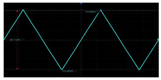
• Y1 -- The upper (default) horizontal dotted line. It can be manually moved to any vertical position on the screen.
