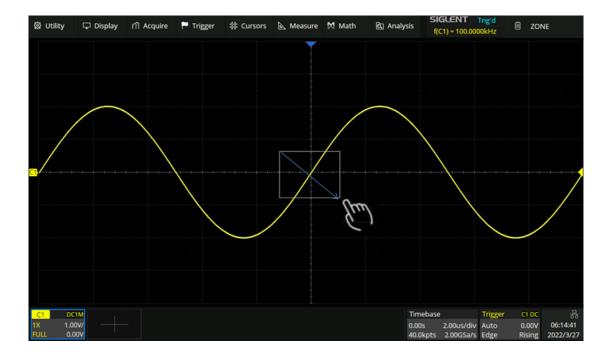
When the finger moves out of the screen, a menu pops up for selecting the zone and setting the zone properties:
