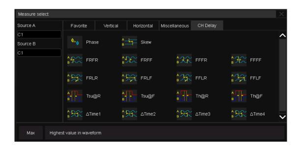
In the parameter selection area, the channel corresponding to *Source A* is specified first, and then the channel corresponding to *Source B*. Finally, the measurement parameter is selected. For example, to activate the skew between C1 and C2, you can follow the following steps:
