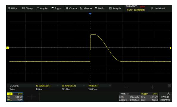
In the example, 74403 pulses can be obtained with the sample rate of 2 GSa/s at the maximum memory depth.
