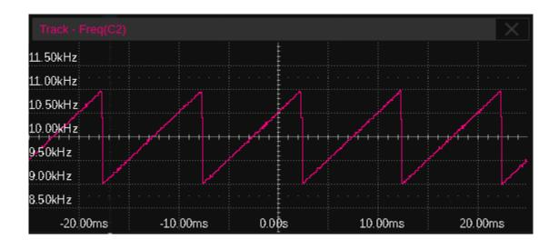
The upper limit of the statistic number in a frame is set in Statistics > AIM Limit, which means the values exceeding the limit will not be shown in the track plot.
