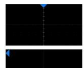
**Trigger Delay Indicator** locates where the waveform triggers on the horizontal axis... When the trigger position is outside the screen, the direction of the triangle points outside the screen as well.
