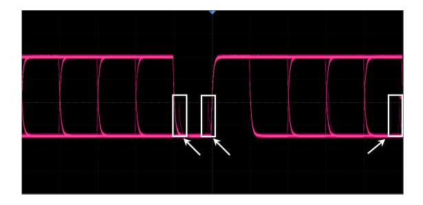
When the display dialog box and persist are off, touch | Display | > Presistencet | can quickly turn on persist.
