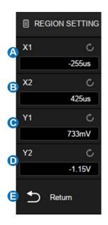
**Note**: If zone1 and zone2 are both turned on, the result of the "AND" operation in two zones becomes the qualified condition of triggering.
