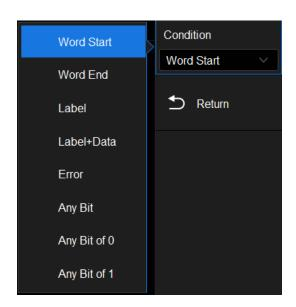
**Word Start** -- The oscilloscope triggers at the start of the word.
