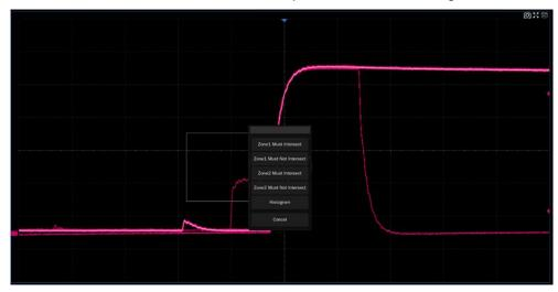
Now, we can accurately capture the exact bus contention waveform:
