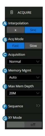
**Interpolation** -- At small timebase settings, the number of original points on the screen may be less than the number of display pixels in the grid area, so interpolation is necessary to display a continuous waveform. For example, at 1 ns/div timebase and 4 GSa/s sample rate, the number of original points is 40, but the grid area includes 1000 horizontal pixels. In this case, the oscilloscope needs to interpolate the original points by 25.
