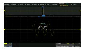
Adjust the horizontal scale of the Zoom window by horizontal pinch and spread in the zoom area of the main window or the Zoom window
