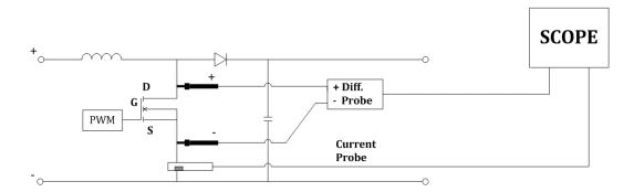
**Note:** Perform a Deskew operation between the voltage and current input channels before the test. See section "Switching Loss" for more details on deskewing.
