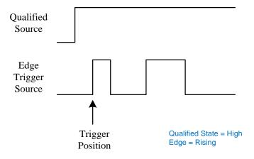
When the type is "Edge", the oscilloscope triggers at the first edge after the specified edge (Rising or
