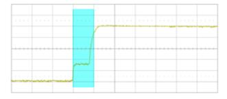
With a simple edge trigger, it is unlikely to trigger consistently on this anomaly. Thanks to the high waveform update rate of the SDS3000X HD, we can confirm there is bus contention happening by
