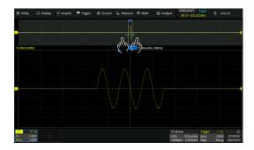
Adjust the horizontal/ vertical scale of the main window by using a pinching or spreading gesture in the gray area of the main window
