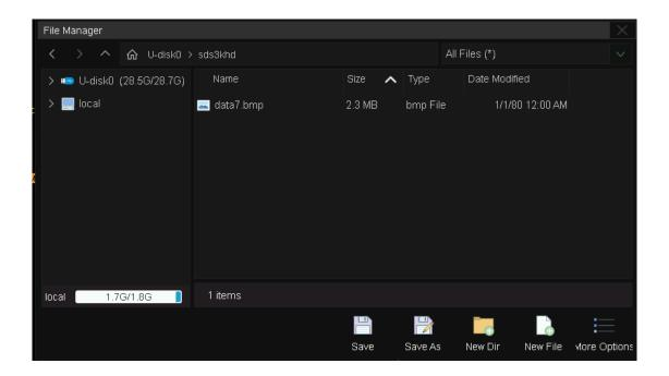
In step 4, if Save is selected instead of Save As , the system saves the file as the default file name SDS3xx4XHD\_BMP\_n.bmp, where n is an integer incrementing from 1. The default save path is \SIGLENT\.
