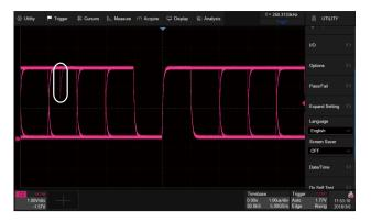
With a waveform update rate of up to 110,000 wfm/s, the oscilloscope can easily capture unusual or low-probability events. In Sequence mode the waveform capture rate can reach 500,000 wfm/s
