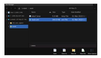
Perform Utility > Screenshot or pressing the Save button (If the function of the button has been defined as "screenshot") to capture the screen to a .bmp\ .jpg\ .png picture. The file will be saved in the path specified in the File Manager.
