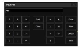
To use the operation of setting "deskew" of the channel as an example: If the expected value is 65 ns, input "65" on the virtual keypad, and then choose the unit n to complete the operation. On the virtual keypad, clicking the button Max, Min, and Default quickly sets the parameter to its maximum, minimum and default values.
