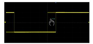
Drag the waveform left and right to move it on the horizontal axis
