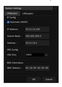
After Connecting to the LAN successfully, the instrument can be remotely controlled by WebServer or by sending SCPI commands via NI-VISA, Telnet, or Socket.
