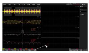
The instrument is able to automatically allocate a trace to a window according to the window layout and traces activated. If the user want to adjust the mapping relationship between a trace and a window, simply drag the Channel Descriptor Box of the trace to the destination window, as the right figure above shown. In this figure F2 is originally shown in window (4,1), to drag its channel descriptor box to window (4,2) will have the trace shown in window (4,2).
