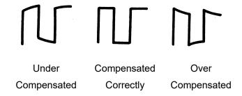
3. Use a nonmetallic flat-head screwdriver to adjust the low-frequency compensation adjustment hole on the probe until the waveform matches the "Compensated Correctly" waveform above.
