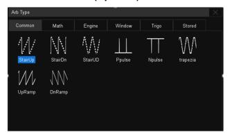
The USB waveform generator can output waveforms with up to 25 MHz frequency and ±3 V amplitude. Six basic waveforms together with multiple types of predefined waveforms and as user-defined arbitrary waveforms are supported.
