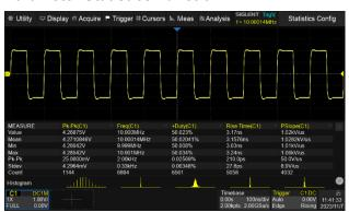
Statistics show the current value, maximum value, minimum value, standard deviation, and mean value. A histogram is available to show the probability distribution of a parameter. Trend and Track are available to show the parameter value vs. time.
