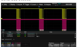
Display the decoded characters through the events list. Bus protocol information can be quickly and intuitively displayed in tabular form. I<sup>2</sup>C, SPI, UART, CAN, LIN are supported.
