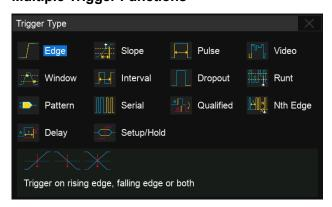
Edge, Slope, Pulse width, Video, Windows, Runt, Interval, Dropout, Pattern, Qualified, Nth edge, Delay, Setup/Hold time, and Serial trigger.
