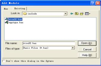
This allows the VISA functions and VISA data types to be used in a program.
