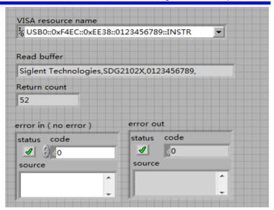
In this example, the VI opens a VISA session to a USBTMC device, writes a command to the device, and reads back the response. In this example, the specific command being sent is the device ID query. Check with your device manufacturer for the device command set. After all communication is complete, the VI closes the VISA session.
