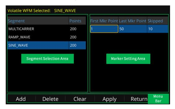
As shown in above figure, the marker setting page is composed of waveform segment selection area, marker setting area and menu bar.
