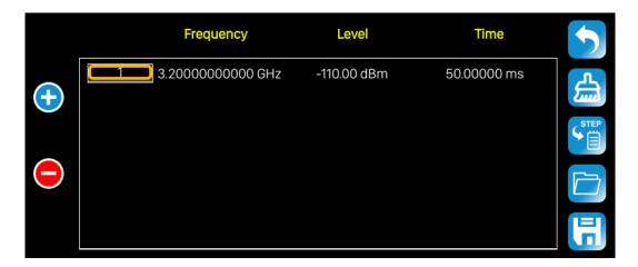
As show in the figure, the table edit page consists of the operating button on the left of page, the table on the middle of the page and the menu button on the right side.
