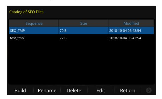
Press **Build** to create a sequence. All operations of creating a waveform sequence can be realized through the touch screen of the signal generator:
