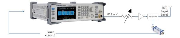
As shown in the example, the sensor measures a proportional power in defined time intervals, derived from a coupler. It considers optionally the given S-parameters and returns the results to the generator. The signal generator compares the measured level with the set value and adjusts its output level accordingly. This allows you to control the external signal level continuously and reliably reach a constant input level at the DUT in real time.
