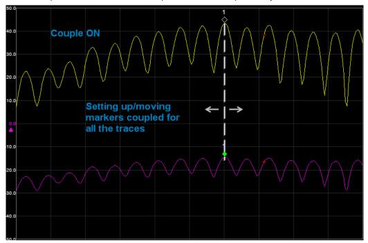
Figure 3-4 Marker Couple is ON
