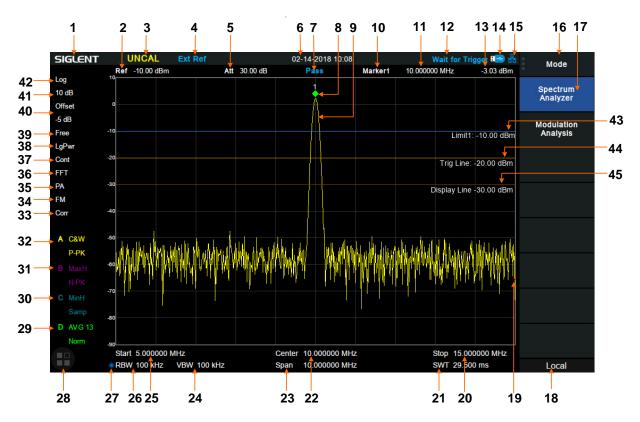
Figure 1-12 User Interface of spectrum analyzer mode
