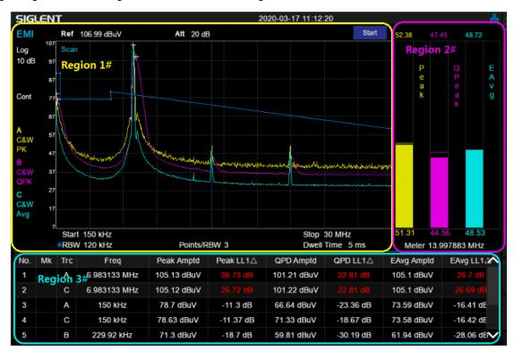
Figure 7-1 EMI Measurement User Interface
