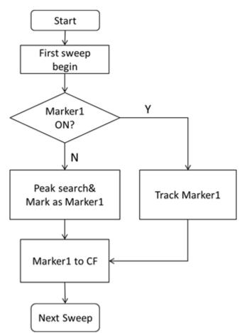
Figure 2-1 Signal Tracking Flow
