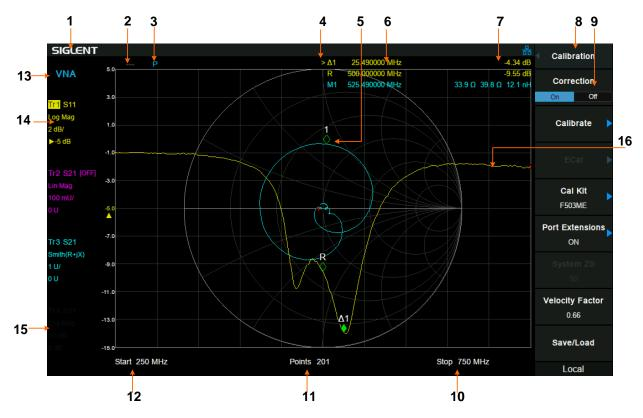
Figure 1-13 User Interface of Vector Network Analyzer Mode
