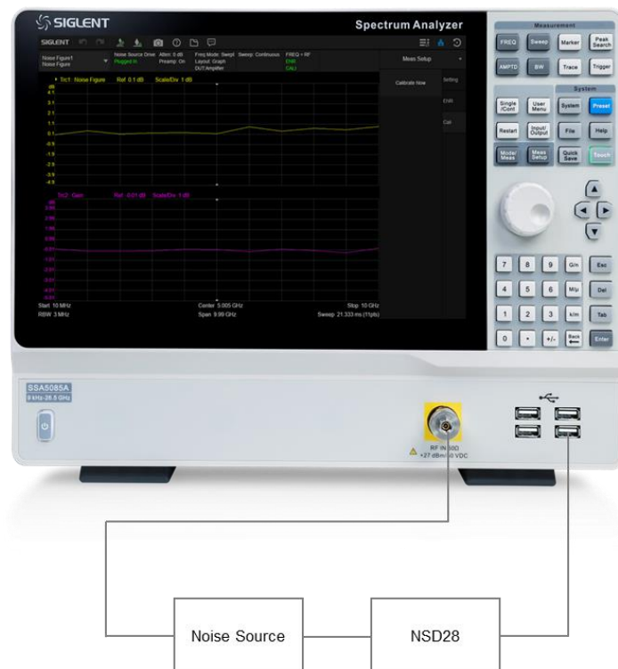
Figure 1-2 Connection setting of noise figure measurement calibration
