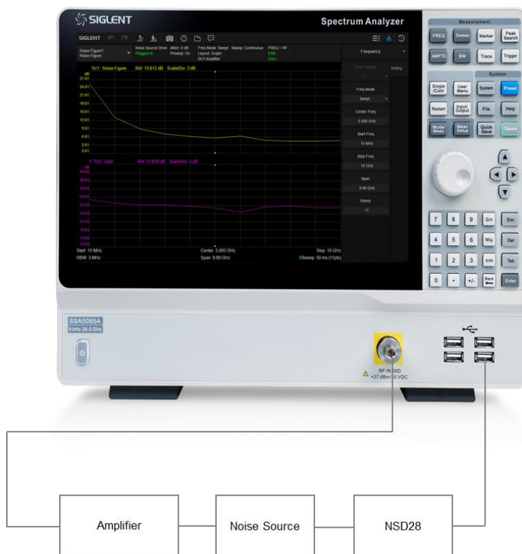
Figure 1-6 Connection settings for noise figure measurement
