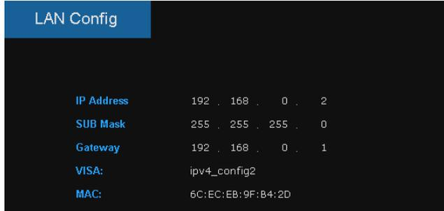
Figure 2-16 Static IP Config
