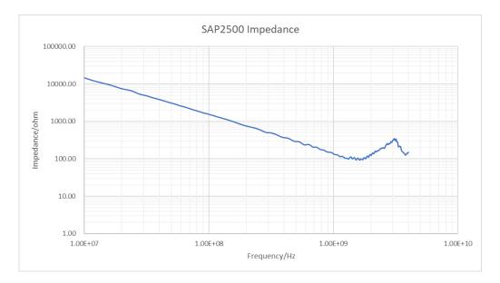
Figure 4 Input impedance over frequency of SAP2500
