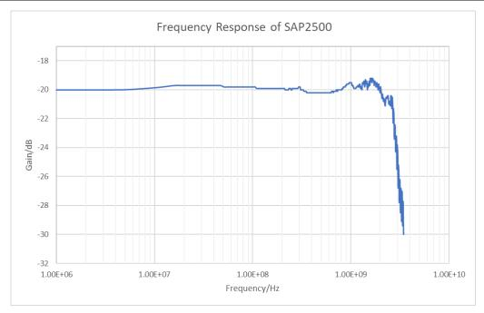
Figure 3 Typical frequency response of SAP2500
