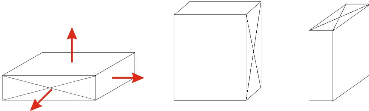
So, whenever attempting to correlate the measurement result, it is necessary to find the DUT orientation, which yields the highest emission levels. There is not necessarily just one single, “worst” orientation. A DUT typically would radiate at various frequencies, originating from different building blocks of the DUT. Consequently, the worst case orientation may not be the same for different spurious.
