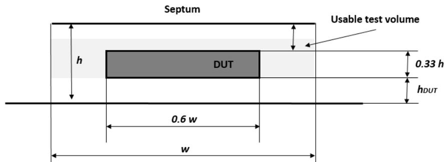
When rotating the DUT into any of the three main orthogonal positions, the geometrical center of the electronic section of the device shall remain in the same position.
