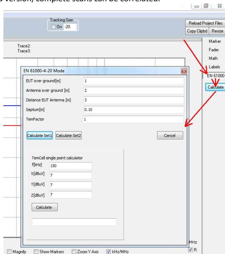
Start the correlation tool by clicking the EN61000 and CALCULATE buttons. In the pop up window, enter the test site parameters according to standard and the septum height of the respective TEM-cell. The TEM-
