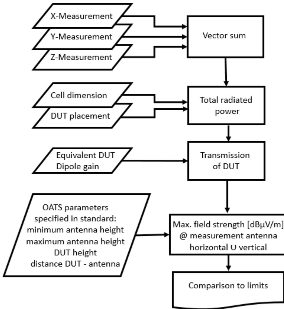
According to IEC 61000-4-20, following requirements with respect to DUT size and placement in relation to the dimensions of the TEM cell need to be fulfilled in order to achieve acceptable accuracy:
