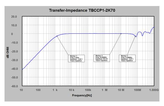
Figure 1: transfer impedance, 10 Hz - 1 GHz, typical data
