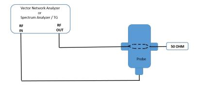
Figure 4: S21, transimpedance measurement set up
