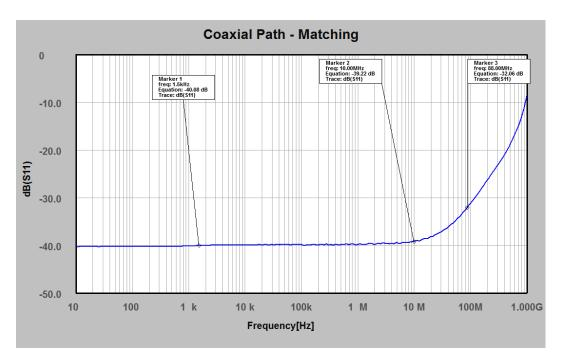
Figure 3: S11, impedance matching of the coaxial path, 10 Hz - 1 GHz, typical data
