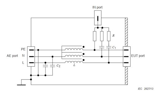
CDN-M3,  $C_1$  (typical) = 10 nF,  $C_2$  (typical) = 47 nF,  $R = 300 \ \Omega$ ,  $L \ge 280 \ \mu\text{H}$  at 150 kHz CDN-M2,  $C_1$  (typical) = 10 nF,  $C_2$  (typical) = 47 nF,  $R = 200 \ \Omega$ ,  $L \ge 280 \ \mu\text{H}$  at 150 kHz CDN-M1,  $C_1$  (typical) = 22 nF,  $C_2$  (typical) = 47 nF,  $R = 100 \ \Omega$ ,  $L \ge 280 \ \mu\text{H}$  at 150 kHz
