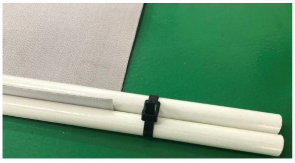
Picture 4: how to tightly roll up the ground plane
