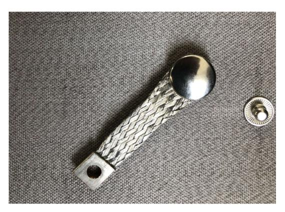
Picture 3: using textile rivets to establish electrical contact to the ground plane
