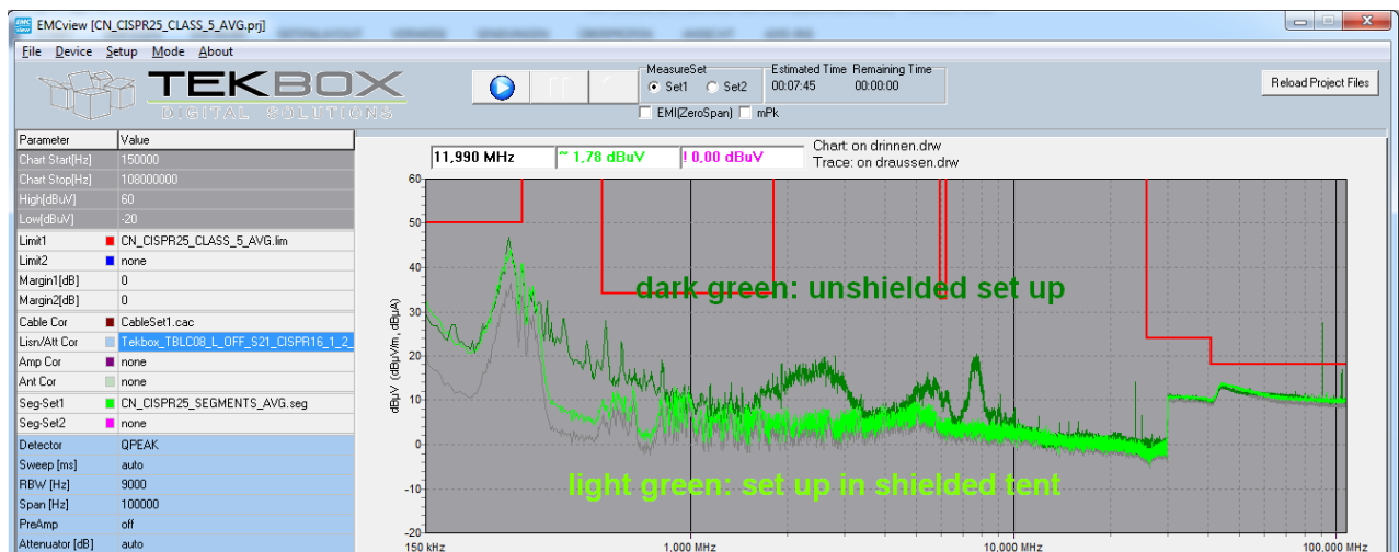
Picture 6: CISPR 25 conducted noise measurement; DUT powered
