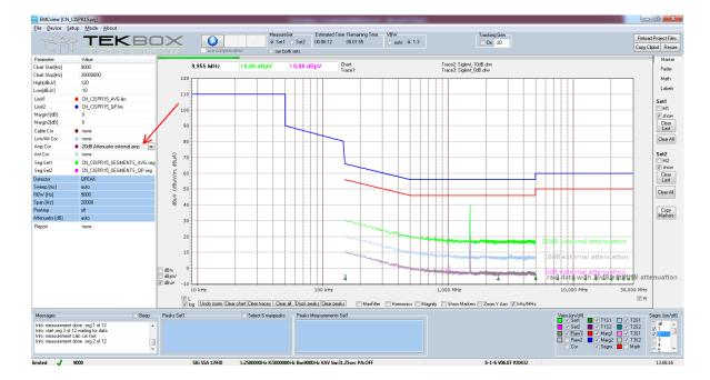
And here the zoomed view. The amplitude values (raw values) obtained from the analyzer are not compensated with respect to the internal attenuation. EMCview compensates the raw values based on the content of the amplitude file.
