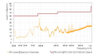
In the legend of the screenshot you can see QP limits, but the measurement was carried out using the peak detector. Peak detector measurement results are far faster than QP measurements and Peak detector measurements always deliver a higher value than QP measurements. As in the above case, the Peak result is not crossing the QP limits, you know that the radiated noise test is passed and there is no need to make a QP measurement.
