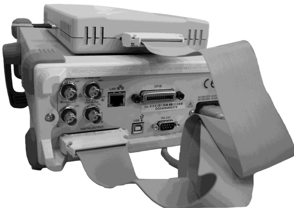
Figure 1-5 Connect the module to DG3000
