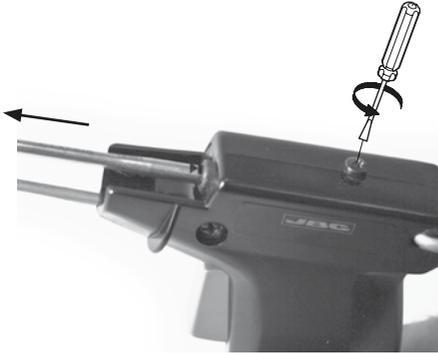
Loosen the screw and remove the cartridge. Use a plier to remove it if still hot. ⚠
