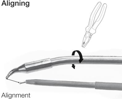
Align the tip of the cartridge with the feeding tube. Use a plier for a safe tip alignment.
