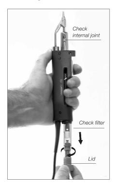
The lid must be removed with the DR560 in vertical position.
