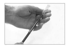
The filter and internal joint must be checked and replaced if dirty or damaged.
