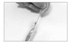
Remove the coil to clean the inside of the deposit with the stick supplied.
