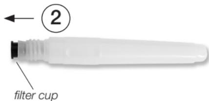
**3.** Completely fill with flux and reseal with the filter cap.
