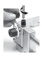
1. Remove the 4 clamp knobs and the 4 black rubber caps.
