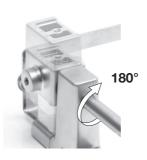
2. After removing both guides, turn 180° the guide supports.
