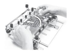
Push the PCB against the SP guide, position it and tighten the SP guide knobs.
