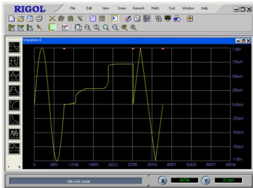
In order to meet the most basic needs of users, UltraWave provides 9 standard waveforms: Sine, Square, Ramp, Pulse, ExpRise, ExpFall, Sinc, Noise and DC. In addition, hand drawing, line (point by point) drawing and arbitrary points drawing are also offered to make it easier to create complex waveforms and to edit multiple waves simultaneously through the multi-file management interface.
