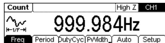
The counter could be used to measure these parameters: frequency, period, duty cycle, positive pulse width and negative pulse width within the range of 100 mHz to 200 MHz.
