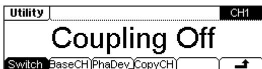
**Channel Coupling:** Once you setup the base channel and the Frequency/Phase deviation of the two channels, the Frequency/Phase of the other one will vary with the base channel and will still keep the deviation you have selected.
