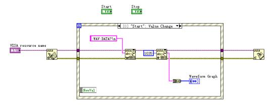
Right-click the "selector label" and choose "Edit Events Handled by This Case" or "Add Event case" to add events respectively for each button. Press "Start" to capture waveform and "Stop" to exit the program.
