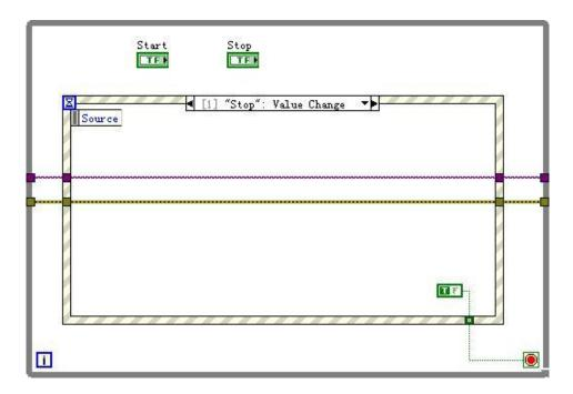
**10.** Change the input tunnel of VISA resource name and errors into **"Shift Register"** to finish creating program.
