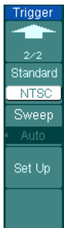
Figure 2-44 Table 2-26 The Video Trigger menu (All lines, Odd field and Even field, Page2/2)
