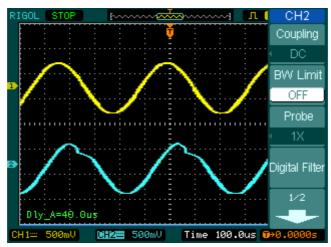
Figure 3-1 Waveform distortion
