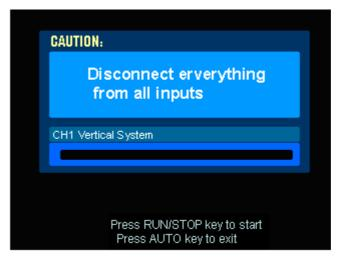
Figure 2-99 The Self-Calibration menu
