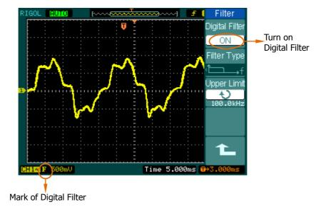
Figure 2-10 Turn on digital filter
