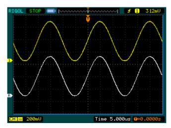
Figure 2-30 Reference waveform display
