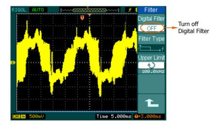
Figure 2-9 Turn off digital filter
