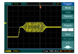
Figure 2-41 Video Trigger: Line Synchronization
