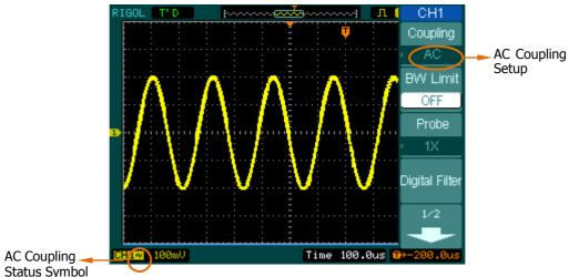
Figure 2-3 AC coupling setting
