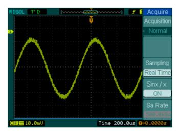
Figure 3-2 Signal with noise
