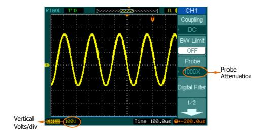
Figure 2-8 Setting probe attenuation
