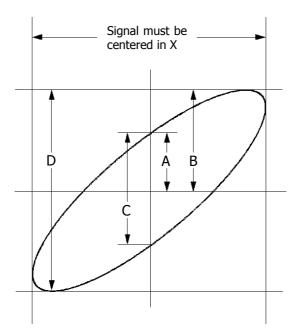
Figure 3-6 Ellipse method to observe the phase difference
