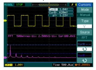
Figure 3-9 Cursor amplitude measurement
