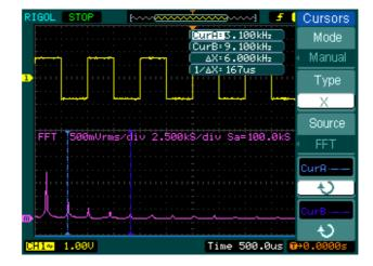
Figure 3-10 Cursor frequency measurement
