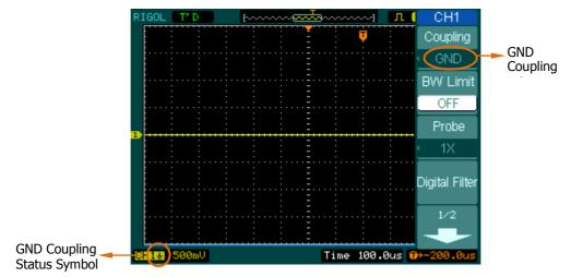
Figure 2-5 GND coupling setting
