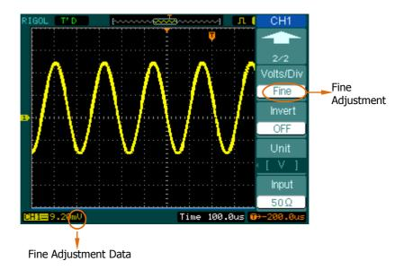
Figure 2-12 Fine configurations
