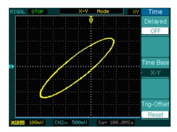
Figure 2-33 X-Y display format
