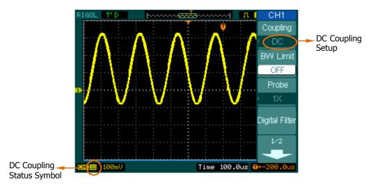
Figure 2-4 DC coupling setting
