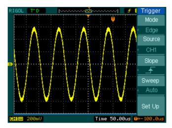
Figure 2-34 Trigger controls
