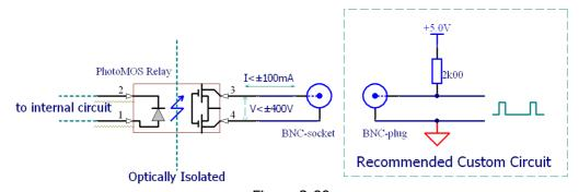
Figure 2-90 Schematic Diagram of Pass/Fail output
