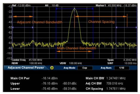
Figure 2-15 Adjacent Channel Power Measurement Interface
