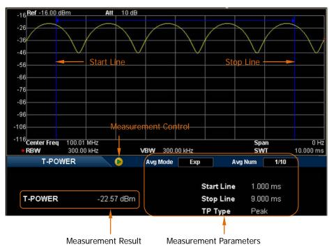
Figure 2-14 T-Power Measurement Interface
