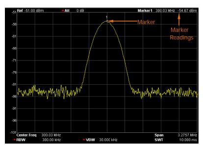
Figure 2-22 Schematic of the Marker
