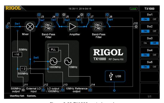
Figure 2-30 TX1000 control panel
