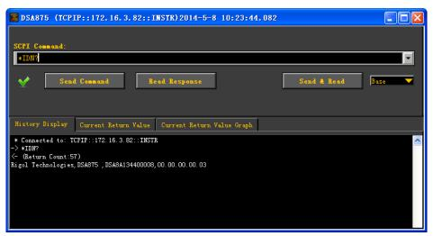
Figure 3-5 Write and Read Commands via LAN
