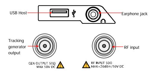
Figure 1-7 Front Panel Connectors
