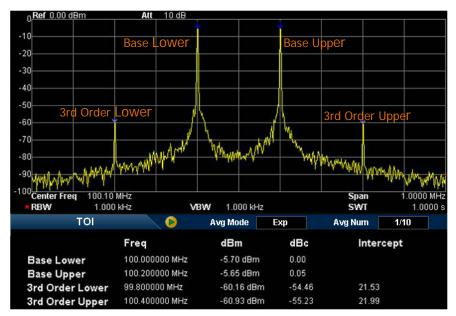
Figure 2-21 TOI Measurement Interface
