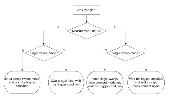
Figure 2-10 Process of Single Sweep
