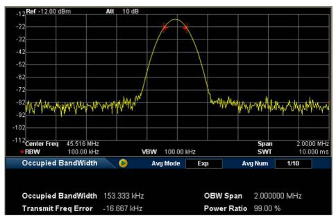
Figure 2-17 OBW Measurement Interface
