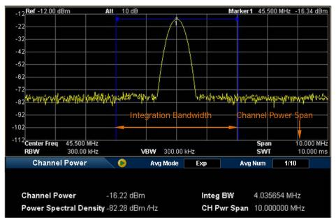
Figure 2-16 Channel Power Measurement Interface
