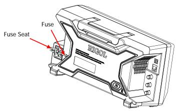
Figure 1-16 To Replace the Fuse
