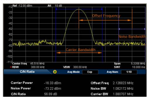
Figure 2-19 C/N Ratio Measurement Interface
