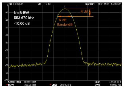
Figure 2-24 N dB BW measurement
