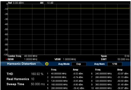
Figure 2-20 Harmonic Distortion Measurement Interface
