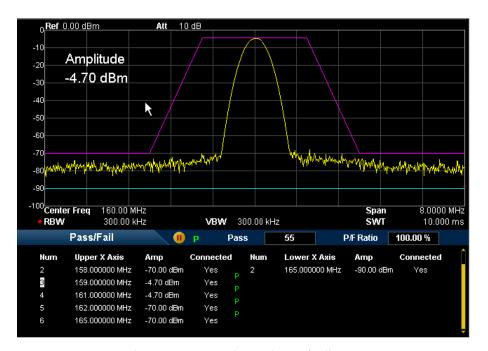
Figure 2-11 Interface of Pass/Fail Test
