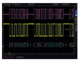
HEX decoded CAN bus signal
