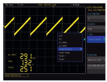
Ramp waveform measured by DVM
