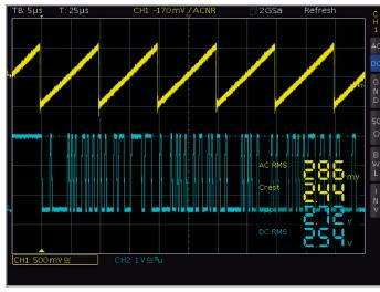
DVM on two analog channels with four measurement parameters
