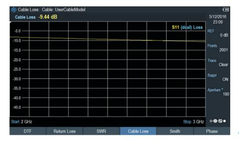
One-port cable loss measurement.
