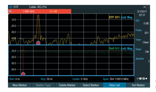
Distance-to-fault measurement and return loss: combined measurement.
