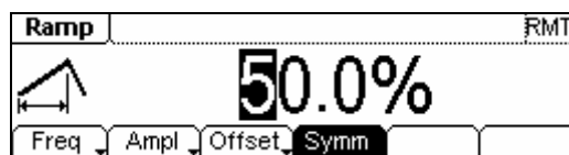
Figure 2-13 The Setting Interface of Ramp Signal
