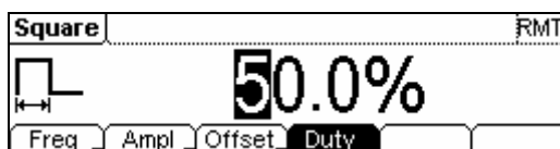
Figure 2-9 The Setting Interface of Square Signal
